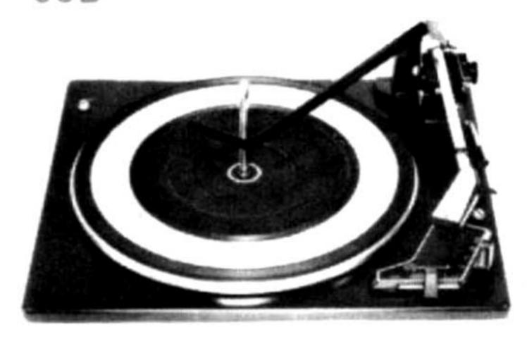
The 401 is a three-speed single record playing transcription turntable for broadcaster and connoisseur alike. Features include illuminated stroboscope, variable speed control (± 3%) balanced and machined diecast turntable, vibration-free operation and fully shielded, shaded four pole induction motor.
