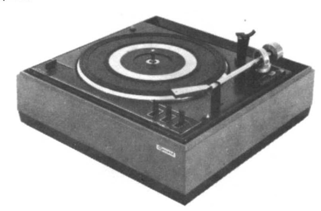
This unit features a weight counterbalanced pickup arm with gimbal type pivots, a slide-in cartridge carrier, integral calibrated stylus force adjustment and bias compensator. For automatic play of single records the easy-to-operate "Auto" tab control is simply moved to "Start" when the arm will position itself on the record and after playing will return to its rest. The unit will then shut off.
