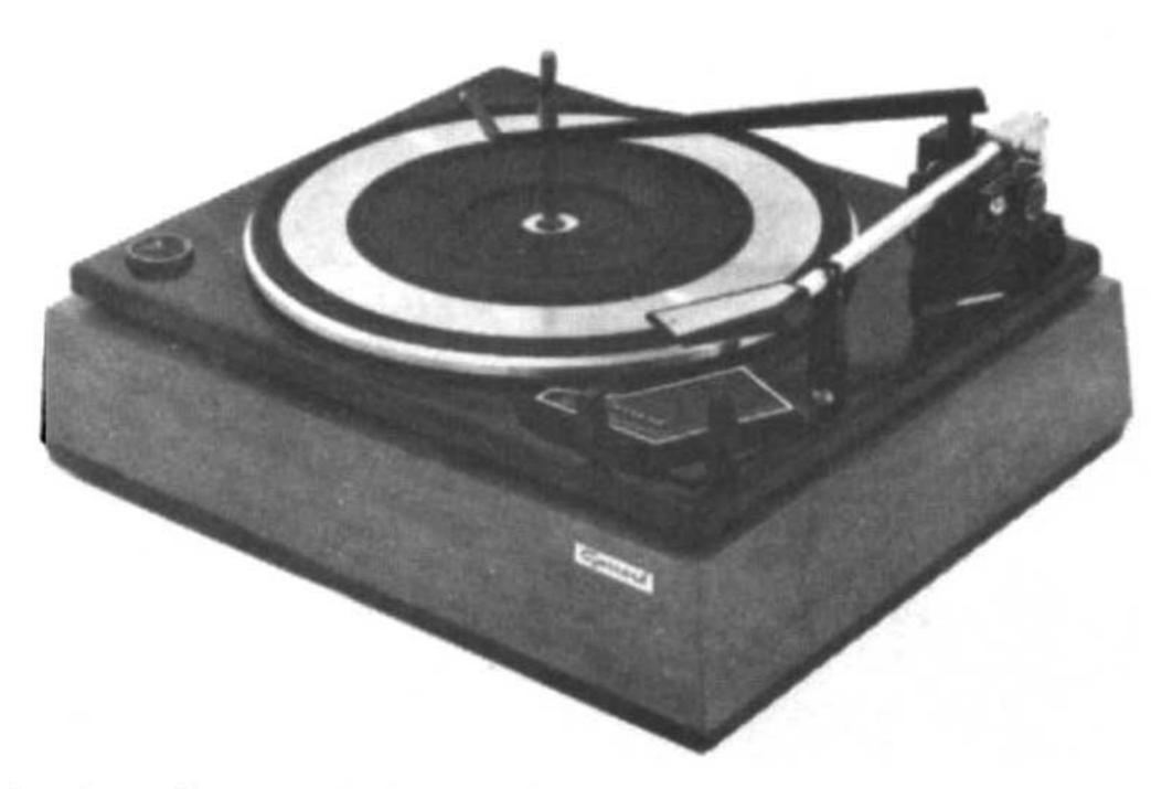
A three-speed automatic record changer fitted with an aluminium turntable and featuring cue and pause control which gently raises or lowers the pickup when the unit is used for playing records singly. The pickup arm is weight counterbalanced and incorporates calibrated fine stylus force adjustment and bias compensation.
